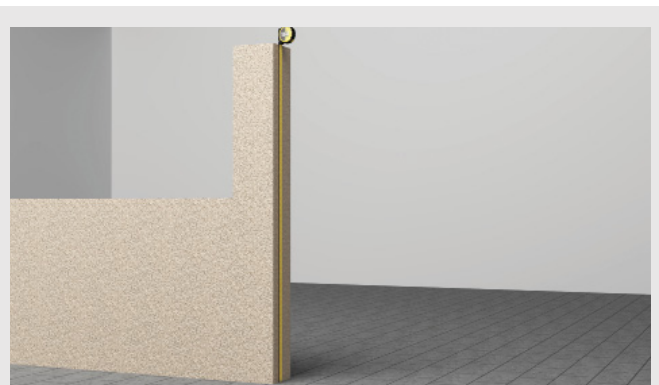
5 Mesurer en haut. Retenir la plus petite mesure; Measure the distance between pillars at the top. Consider the smallest distance (bottom, middle, top);
